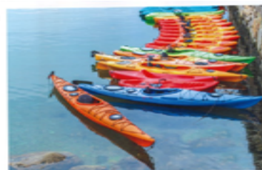
▲ Canoes made from reinforced GRP
