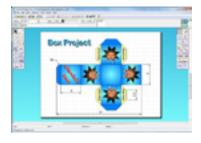
2D CAD soft ware such as Techsoft 2d design can be used to design products such as packaging nets or panels for products. These can then be printed out or laser cut, then made into products.
